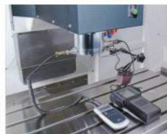
主轴噪声和振动检查 Spindle noise and vibration checks
